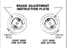
A DRUM BRAKE ASSEMBLY is furnished on our winches to retard the speed of the cable drum when spooling off loose cable. Use of the brake in "free-spooling" of the cable drum prevents tangling of the cable on the drum.
